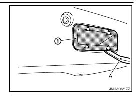
Insert remover tool (A) between back door lower finisher inner
