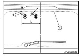
Insert a needle or similar object (B) into the spray opening (A) and move up/down and left/right to adjust the spray position.
